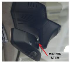
5 - While sitting in the passenger seat, place the mount over the mirror stem. Tighten the CLAMP SCREW until the mount starts to clamp onto the mirror stem. Position the mount as far forward as it will go and paralell to the bottom of the mirror before fully tightening.
