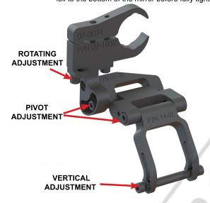
7 - Reinstall the body assembly. Be sure to include all lock washers with screws, and the lock and flat washer with the bottom socket head screw as shown above. Use the adjustments shown above to adjust the RD to your desired position. We recommend adjusting the RD as close to the bottom of mirror as possible. Be sure to tighten all screws after adjustments are made.
